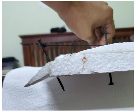
Both pictures illustrate the deflection of the ailerons. (Taken at V's residence)
