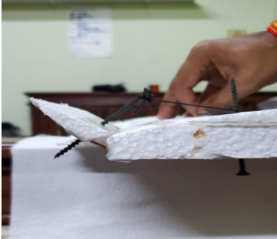
Both pictures illustrate the deflection of the ailerons. (Taken at V's residence)
