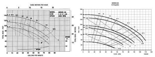
Figure 2. Typical centrifugal pump curves. (MP Pumps, 2017)
